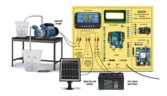
This trainer has been designed with a view to provide practical and experimental knowledge Sensors programing for IoT based Solar Pump with Arduino IOT Board.
